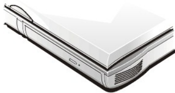
Figure 2. DVD-ROM or CD-ROM Drive Installed in Computer
