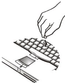
Figure 6. Removing the Track Stick Cap
