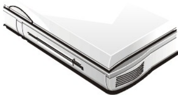
Figure 1. Diskette Drive Installed in Computer
